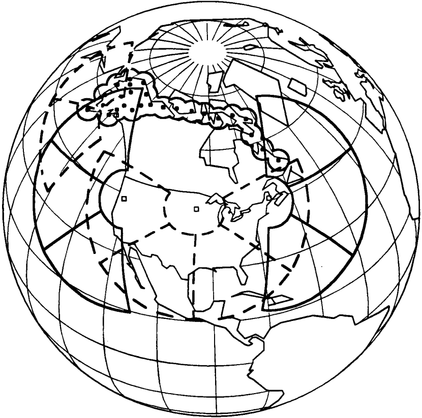
Figure 4: Radar coverage of the planned US 12 sector OTH-B system. Sectors shown with dashes were planned but have not been built. Also shown (circles) is the high-altitude coverage of the 15 long-range FPS-117 radars of the North Warning System. The high-altitude coverage of the FPS-117 radars of an Alaskan radar system known as SEEK IGLOO is also shown.
