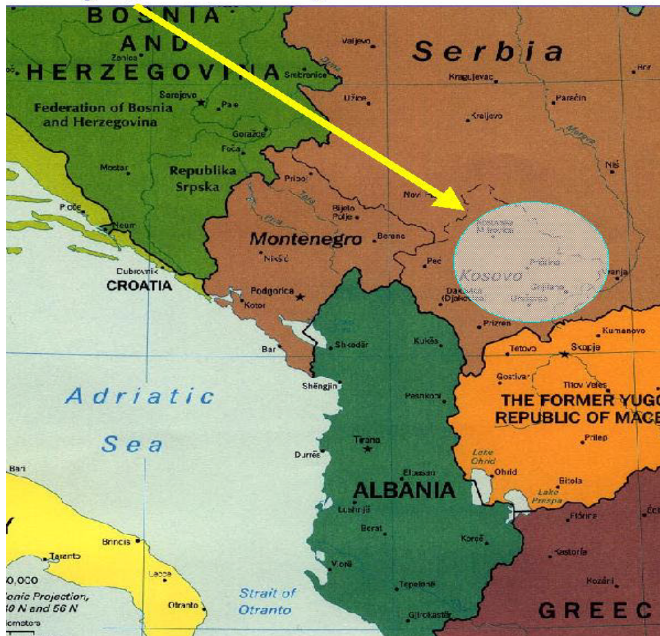
Figure 4: Simulating 1000 Tomahawk missile attacks against Pristina. Each missile is assumed to carry 400 kg of DU (worst-case scenario). The downwind isodose radius of the Gaussian model is rotated to cover a 360° potential-hazard zone. Outside the circular zone (50 km), the CEDE will be lower than that of a pelvis x-ray (46mrem).
