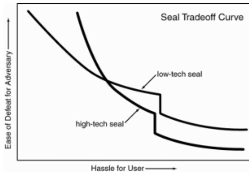
**Figure 3:** Typical tradeoff curves for low-tech vs. high-tech seals (including seals that use high-tech readers). While the high-tech seal can provide better tamper-detection, you often must actually do more work, not less, to achieve the higher security.
