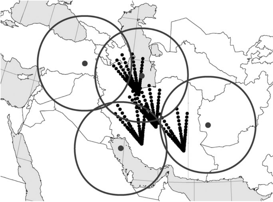
Figure 19: ABI intercepts against 240-sec liquid-propellant Iranian ICBMs.
