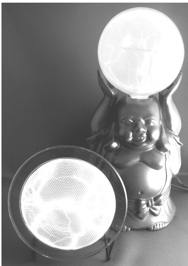
Figure 4: A consumer 2-dimensional Lumina Disk, left, and a 3-dimensional Buddha Spherical Lamp, right, of questionable taste. These are sold to consumers as retail novelties and decoration for approximately $19 and $25, respectively. The plasma discharge “fingers” that each device generates fluctuate unpredictably in time and space. Up to 4 different photosensors, if sufficiently spaced, can measure the light levels at different points on each device without any significant correlation or anti-correlation in their measurements.
