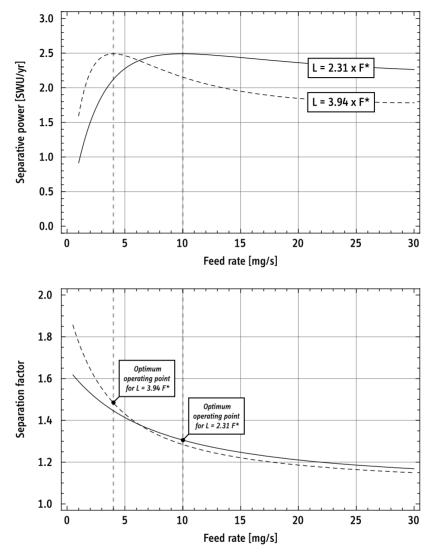
**Figure 3:** Separative performance of a P1-type machine as a function of the feed rate for fixed internal circulation (top). Values for the countercurrent rates L have been chosen such that  $\delta U$  is maximized for 10 mg/s (P1-100) and for 4 mg/s (P1-040). These design points are used for an analysis of cascade-performance below. The respective separation factors are also shown (bottom). Results based on the analytical model by Rätz using Eq. (10).
