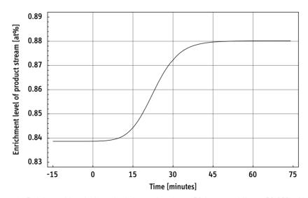
**Figure 4:** Enrichment level of product stream leaving a P1-type centrifuge (P1-100). At t=0, the feed rate is gradually reduced from its reference value of 10 mg/s to 5 mg/s over a 30-min period. The separative performance drops slightly from its optimum value (2.5 SWU/yr) to about 2.3 SWU/yr, if the internal circulation is not adjusted. A new equilibrium is obtained within about one hour. In this simulation, the feed material is natural uranium, and the cut is 0.46.
