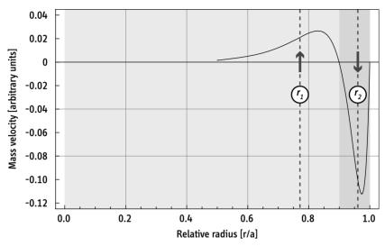
Figure 1: Typical mass-velocity profile expected for a centrifuge.
