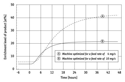
**Figure 6:** Transient response of a 164-machine cascade using P1-type technology: Enrichment level of product in batch recycling mode, initiated at t=0. Depending on the selected default feed rate, a new equilibrium is reached within 24–48 h.
