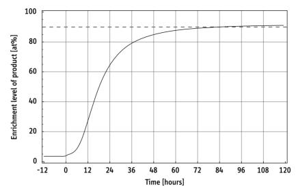
**Figure 7:** Enrichment level of the product recovered from a 164-machine cascade of the second batch recyling step. The machines in this cascade are operated at a reduced flow rate (P1-044); feedstock is 16.3% preenriched material from a first batch recycling step, in which machines are operated at the standard flow rate (P1-135). In this simulation, the target enrichment level of 90% is reached after about 3.5 days.
