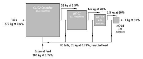
**Figure 8:** Illustration of the cascade arrangement as proposed for the Libyan enrichment project. Note the asymmetric upstream and downstream connections. Mass values are normalized to one kilogram of product (weapon-grade uranium at 90% enrichment), which is produced in about 4.1 days with this setup, if based on P1-type technology.
