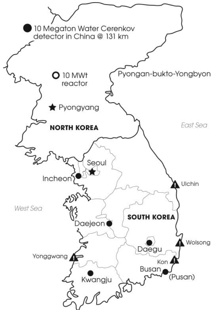
Figure 18: A hypothetical deployment sensitive to a 10 MWt in Yongbyon, North Korea. The size of the detector (or array of detectors) is 10 megaton. A 1 year dwell time would achieve an 8 sigma measurement of a 10 MWt reactor at the indicated location. Included in the calculation are backgrounds from all South Korean reactors, with sites in South Korea indicated by the triangles, as well as detector related internal and external backgrounds, using a rate per unit mass extrapolated from the KamLAND experiment.
