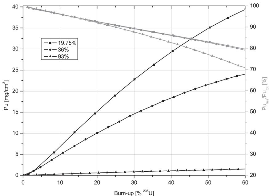
**Figure 2:** Concentration of plutonium as well as fissile plutonium fraction as function of burn-up for three enrichment levels for IAEA’s generic MTR.
