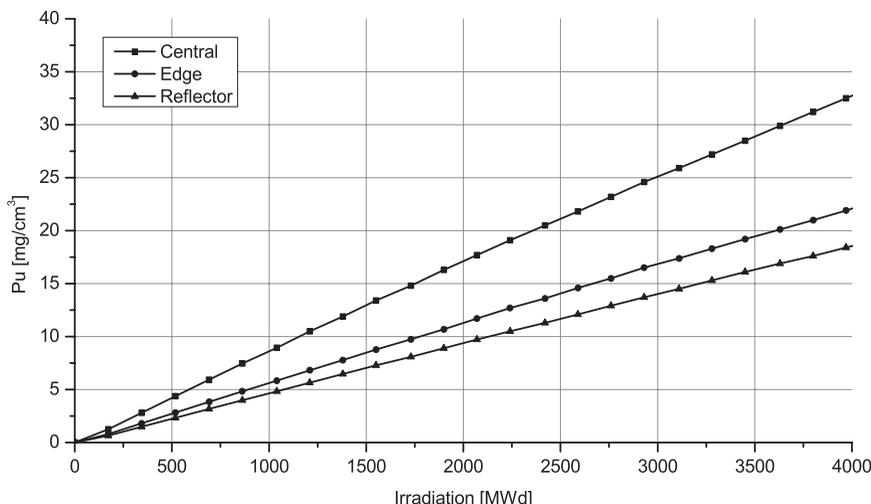
**Figure 3:** Plutonium production in NU-targets in central, edge, and reflector position (scenario B) for 19.75 percent enriched driver fuel. The concentration given for the reflector positions are averaged over all positions.
