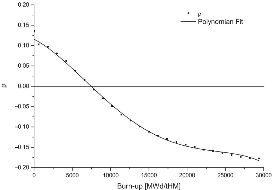
**Figure 4:** Reactivity as function of burn-up for the modeled fuel cell of Arak HWR. The coefficients for the polynomial fit are:  $\rho_0 = 0.116$ ,  $A_1 = -9.60 \cdot 10^{-6}$ ,  $A_2 = -1.38 \cdot 10^{-9}$ ,  $A_3 = -8.92 \cdot 10^{-14}$ ,  $A_4 = -1.46 \cdot 10^{-18}$ .
