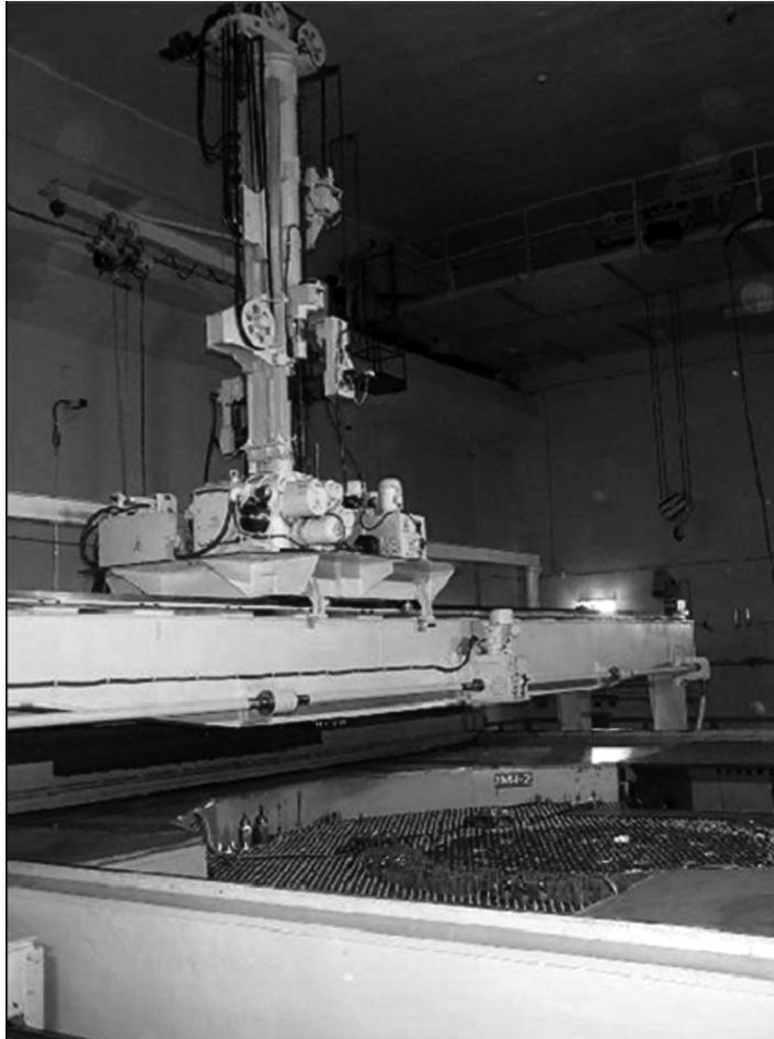
**Figure 1:** The BFS-2 critical facility. The machine above the critical assembly is used for placing and removing fuel assemblies and tubes.
