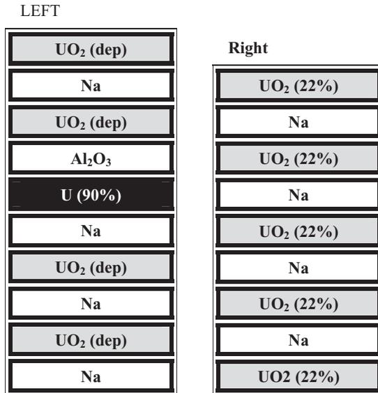
**Figure 2:** An example of a simulation of approximately 18% HEU fuel with a mix of current 90% HEU disks and disks of depleted uranium (left) and 22% HEU (right).
