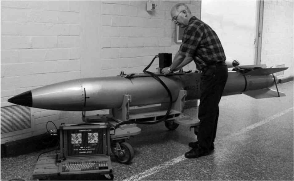
Figure 10: Photograph of the UIT unit used to scan a component.
