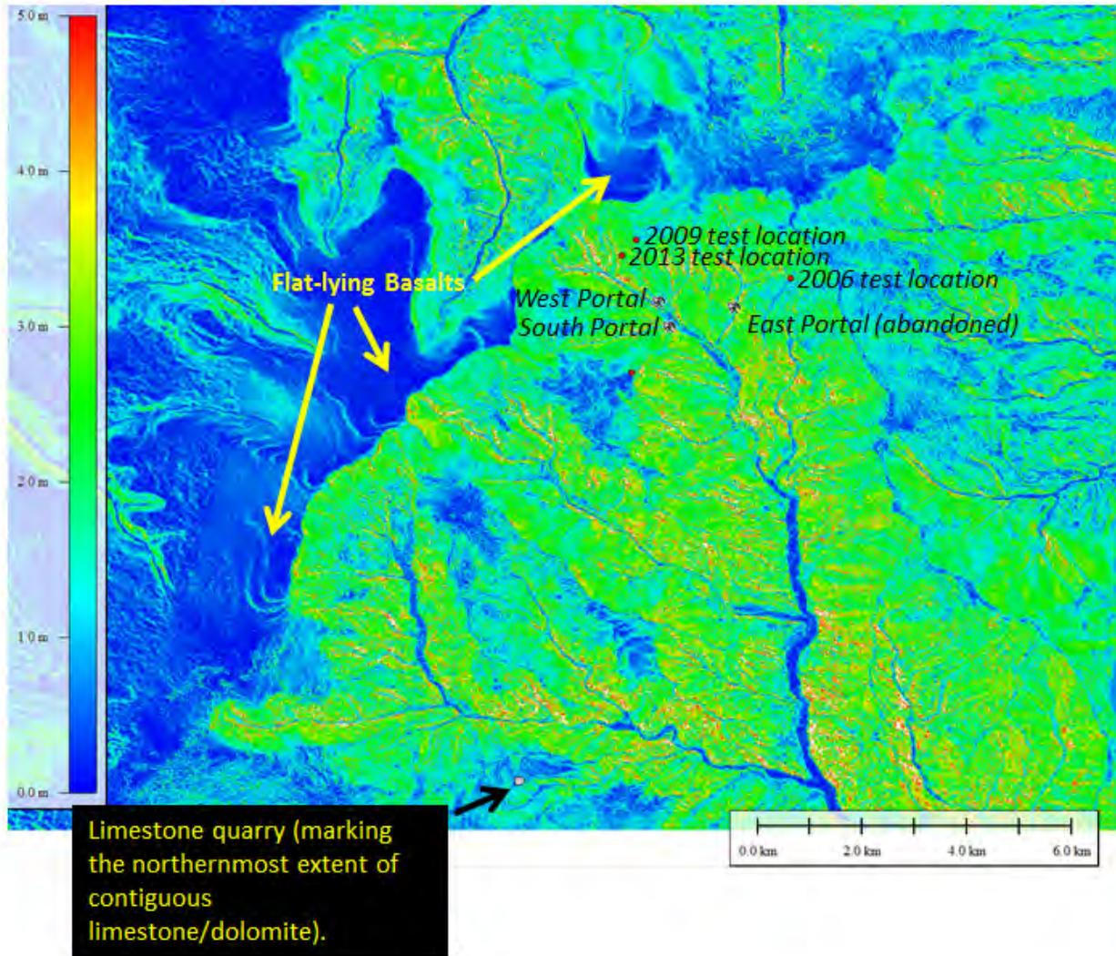
Figure A4: Rugosity (topographic roughness) of the Punggye-ri nuclear test site. Rugosity is calculated from the elevation data and algorithmically derived near neighbor grid comparisons
