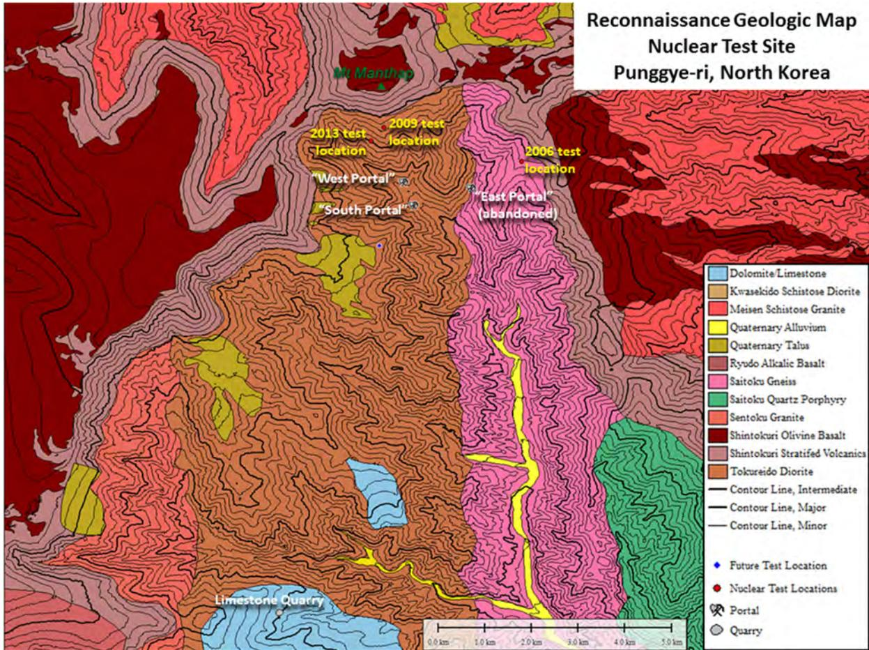
Figure A8: The derived local large-scale geologic map of the Punggye-ri nuclear test site.
