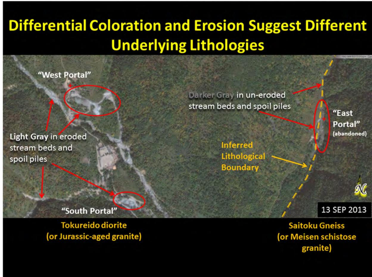
Figure A12: Differential coloration of excavated spoils at the tunneling locations of the Punggye-ri nuclear test site. Coloration variations and differential erosion across the inferred lithological boundary provide additional evidence of different underlying host-rocks.
