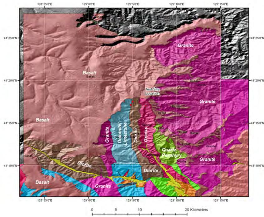
Figure A1 Lower: USGS reconnaissance based geologic interpretation (incorporating ASTER spectral data).
