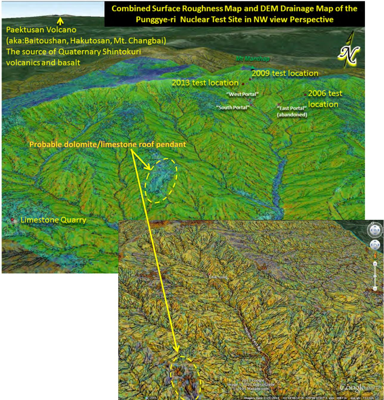
Figure A6: A combined rugosity (surface roughness) map and drainage map for the Punggye-ri nuclear test site. Upper: The derived stream drainage map is shown in perspective on Google Earth. The probable dolomite/limestone "roof pendant" stands out in the lower left center of this combined image. Lower: Terrain types overlain on drainage map, again showing the unique cohesive qualities suggestive of a dolomite/limestone "roof pendant" inside the yellow oval.
