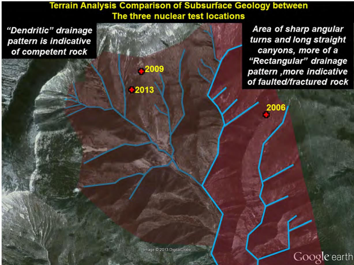
Figure A3: Subjective manual terrain analysis with respect to the openly identified event locations for the three North Korean underground nuclear tests conducted to date. The drainage pattern suggests a differential stream pattern consistent with two different rock types along a lithologic boundary as inferred and mapped by the USGS and separating the two types of host rock associated with underground nuclear testing.
