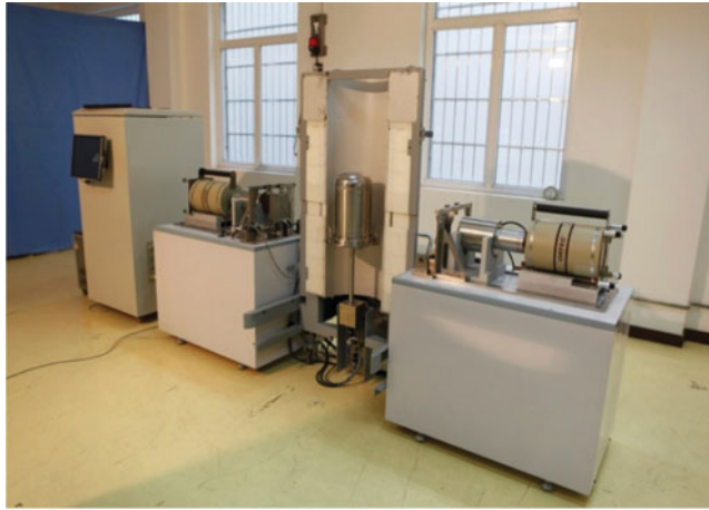
Figure 1: A Pu-subassembly attributes and measurement system with information barrier. © Institute of Nuclear Physics and Chemistry in China Academy of Engineering. Reproduced by permission of Institute of Nuclear Physics and Chemistry in China Academy of Engineering. Permission to reuse must be obtained from the rightsholder.
