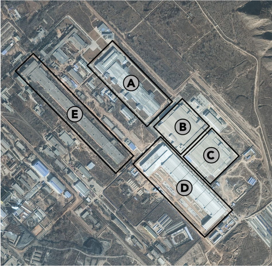
Figure 1: Lanzhou uranium enrichment plant. Label A: Lanzhou CEP 1 (Russian-supplied phase III); B: Lanzhou CEP 2 (Indigenous, demonstration project); C: Lanzhou CEP 3 (Indigenous); D: Lanzhou CEP 4 (Indigenous, under construction); E: Gaseous Diffusion Facility. Satellite image from 18 January 2015 (Coordinates: 36°08'53.30" N/103°31'24.49" E). © DigitalGlobe. Reproduced by permission of DigitalGlobe. Permission to reuse must be obtained from the rightsholder.
