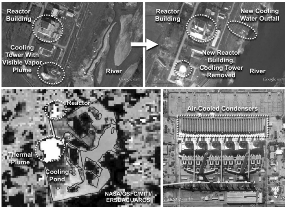
Figure 1. Examples of cooling systems and ultimate heat sinks: steam plume from a cooling tower (top left) 3 ; the same site after removal of the cooling tower, construction of new reactor, and a possible cooling water outfall (top right) 4 ; infrared image of a power reactor and its cooling water pond (bottom left) 5 ; the Matimba Power station, a 4GWe coal power plant – the world’s largest direct dry-cooled power plant (bottom right) 6 ; additional annotations by authors.
