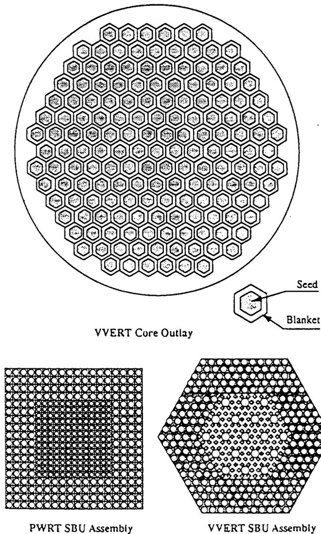
Figure 2: VVERT core outlay and SBU geometry.
