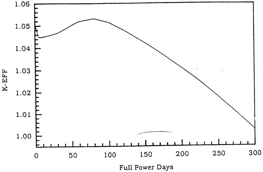
Figure 4a: Core criticality—cycle 5.
