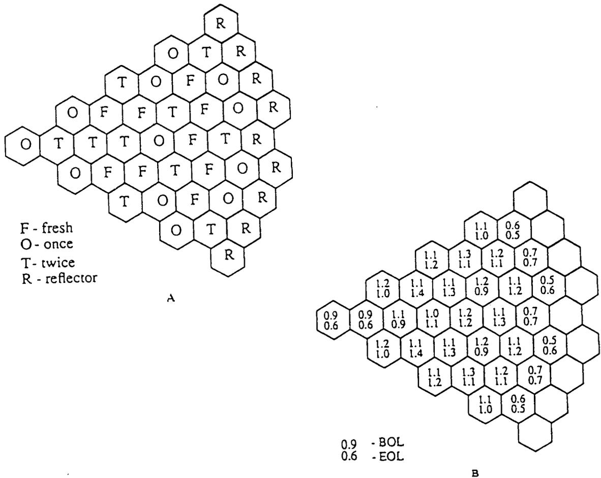
Figure 3: VVERT reload pattern (A) and power distribution (B).
