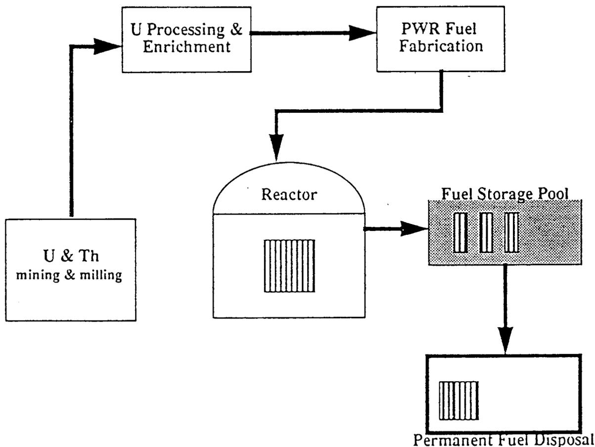
Figure 1: LWR fuel cycle stages without fuel reprocessing.
