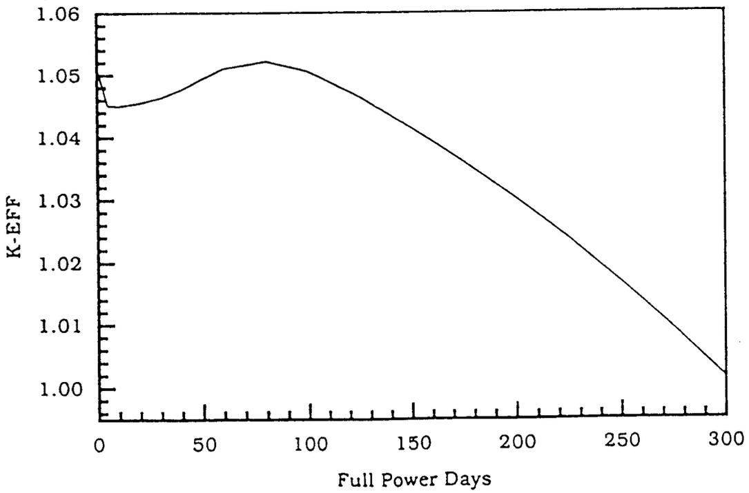
Figure 4b: Core criticality—cycle 6.
