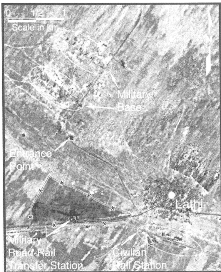
Plate 8: March 25, 1995 SPOT panchromatic image showing area 1 (see plate 7). Although the spatial resolution of the image is relatively low, it was possible to determine the functionality of several structures in the image by identifying distinct features and linking them together through deductive reasoning.
