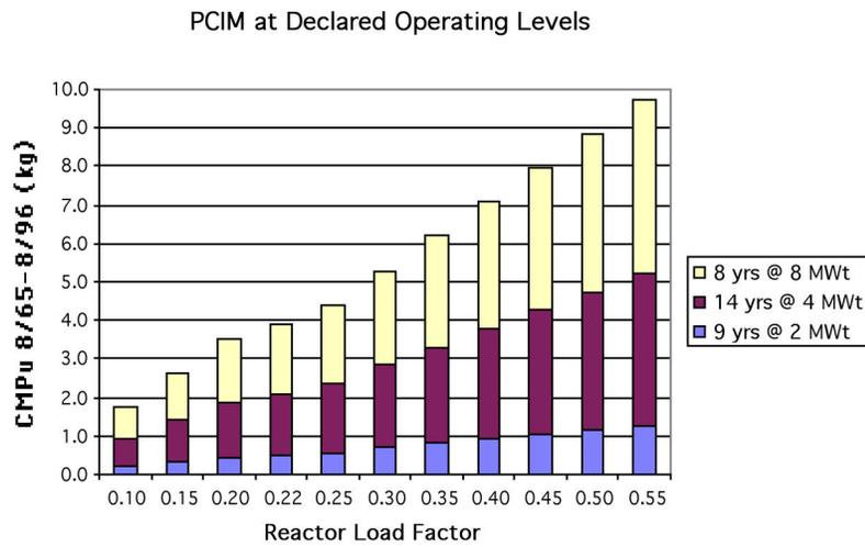
**Figure 1:** IRT-DPRK cumulative maximum PCIM production for declared ( $CMPu_D$ ) power levels, assuming reactor load factors ranging from 0.1 to 0.55, including 0.22 for entire 31 years.
