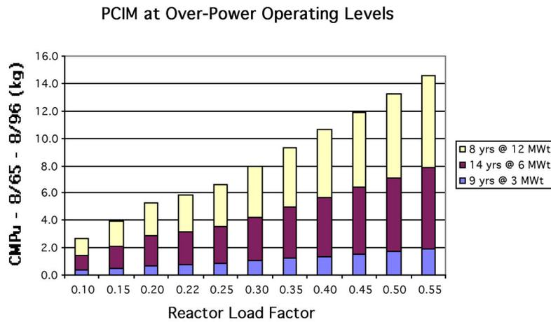
Figure 2: IRT-DPRK cumulative maximum PCIM production for over-power ( $CMPu_{Op}$ ) levels, assuming reactor load factors ranging from 0.1 to 0.55, including 0.22 for entire 31 years.
