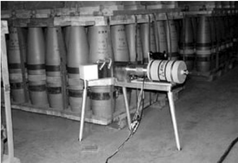
Figure A1: Pallets of 155 mm projectiles each containing approximately 3 kg of GB nerve agent (Sarin) at the Tooele Chemical Agent Disposal Facility in Utah. The munitions are cast from high-strength steel. Prior to incineration, the projectiles are opened with remote cutting tools and the explosive burster removed. Even at incinerator temperatures exceeding 1000°C, full containers of GB require nearly an hour or more to completely vaporize and destroy the agent. The mechanism in the foreground is part of an experiment to develop a method of noninvasive agent identification using neutron spectroscopy. Source: Helmuth, L., Seeing Through Steel: INEEL-Developed Technology Identifies Chemical Weapons . Available at http://www.eurekalert.org/pub_releases/1998-10/INEE-STSI-141098.php (accessed April 1, 2004).
