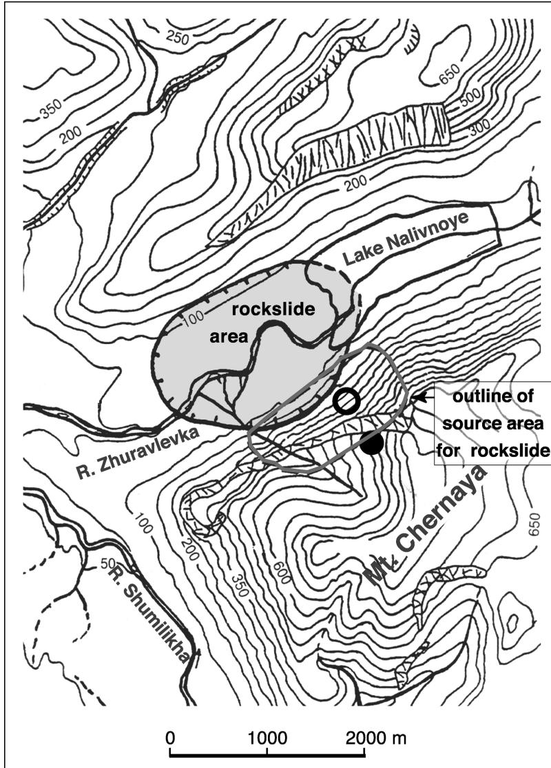
**Figure 6:** A topographical map (from ref. 13, English edition) of the region above the UNT of 12 September 1973. The contour interval is 50 m. The beginning (source) and ending areas of the rockslide are outlined. Filled circle—chambers KB-1 and KB-4; open circle—end of the line of least resistance (LLR), emergent at the surface from KB-4.
