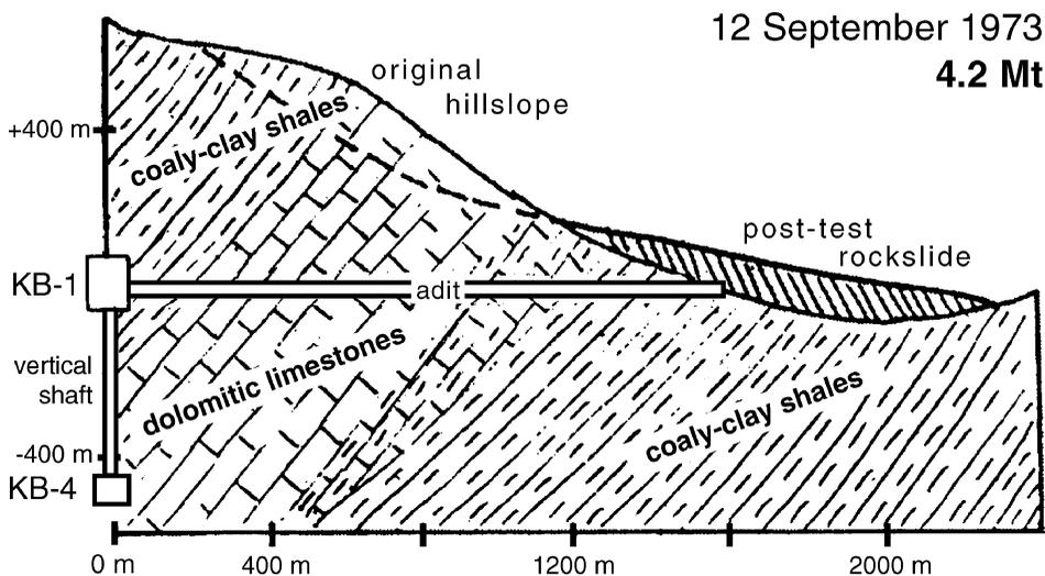
**Figure 5:** A vertical schematic cross-section (based on ref. 14) of the adit-shaft combination of the UNT of 12 September 1973, indicating the position of chambers KB-1 and KB-4. The mountainside is shown before and after the landslide caused by the explosion.
