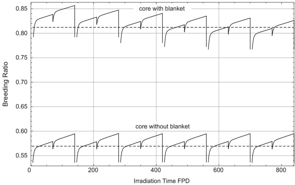
**Figure 4:** Average and time dependent conversion ratios for BN-800 with and without breeding blankets during equilibrium cycle. Two subsequent fuel element cycles are shown to account for a full blanket irradiation. Graphs are cut off below selected values to increase clarity.
