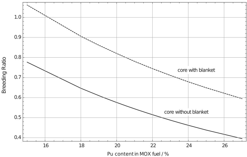
**Figure 5:** Conversion ratio over different plutonium fractions in the fresh fuel.
