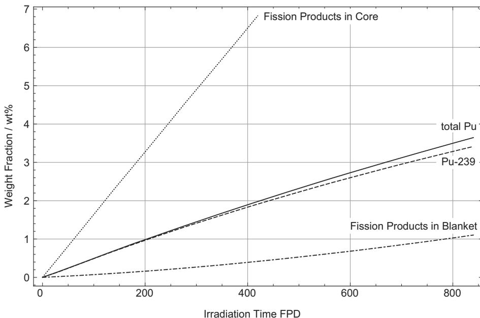
**Figure 3:** Plutonium and fission product content in the radial breeding blankets over time as fractions of the total heavy metal inventory. The solid and dashed line show the plutonium-239 and the total plutonium content respectively. The accumulation of fission products in the breeding blanket is given as well (-.-). For comparison the dotted line shows the fission product content in the fuel of the reactor core without blankets (··).
