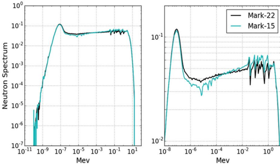
**Figure 2.** Neutron flux spectrum in the outer sleeves of the MARK 22 and the MARK 15. The plot on the right shows the thermal, epithermal, and resonance regions of the spectra.
