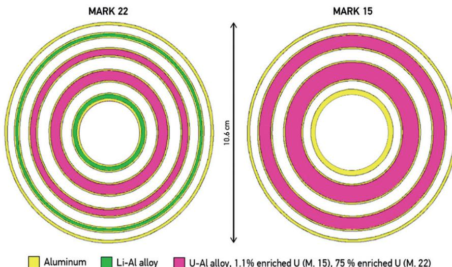
**Figure 1.** Cross-sectional view of Savannah River Plants' MARK 22 assemblies (for tritium production) and MARK 15 assemblies (for plutonium production).
