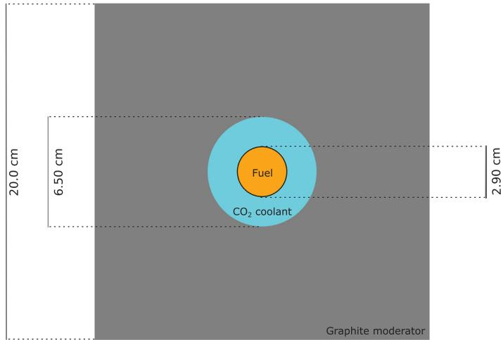
**Figure 2.** Geometry of the unit cell of the 5-MWe reactor. The natural uranium fuel is in orange, the CO<sub>2</sub> coolant in cyan and the graphite moderator in dark gray. The cladding is displayed as a thin line around the fuel.
