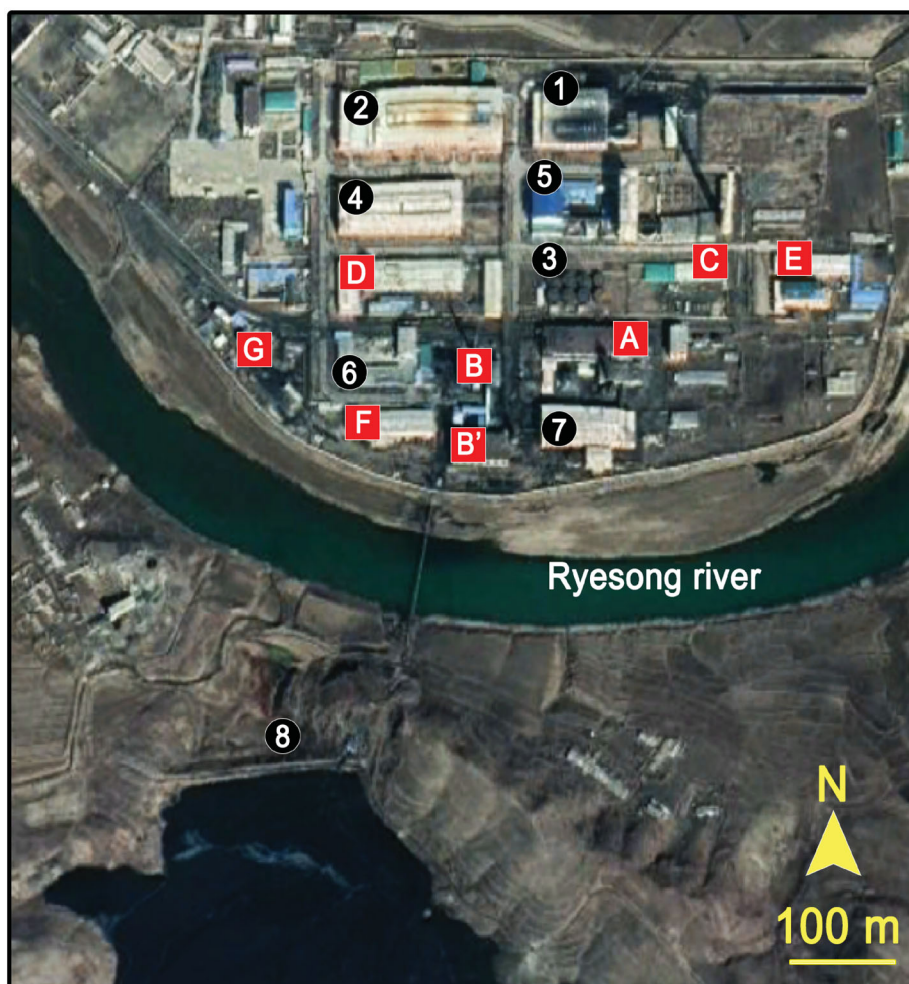
Figure 5. A satellite image of the Pyongsan Uranium Concentrate Plant. Labels 1–8 are buildings and structures directly involved in the uranium to yellowcake pathway. Labels A–E are features that are assumed to be support buildings. Source: Google Earth.
