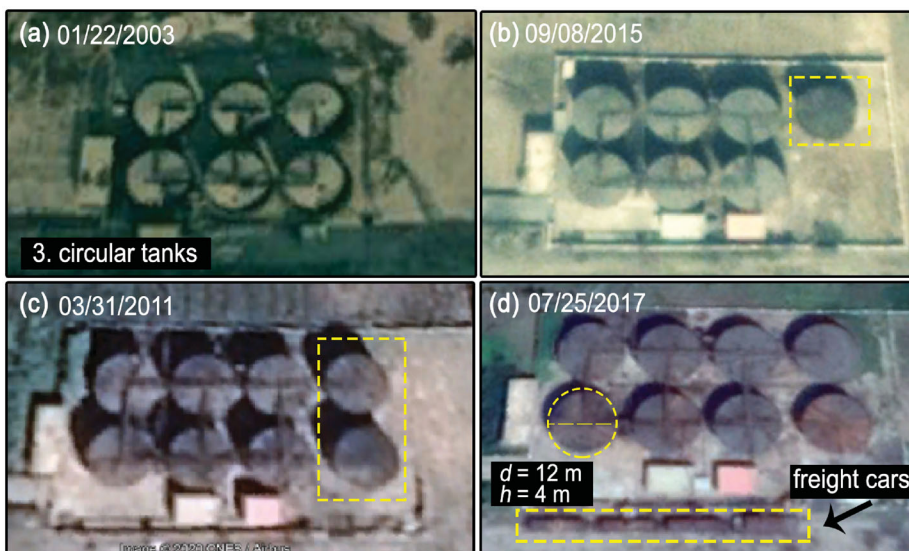
Figure 8. (a–d) Circular tanks at Pyongsan in 2003. Two additional tanks of comparable size were added between 2003 and 2015. Source: Google Earth.
