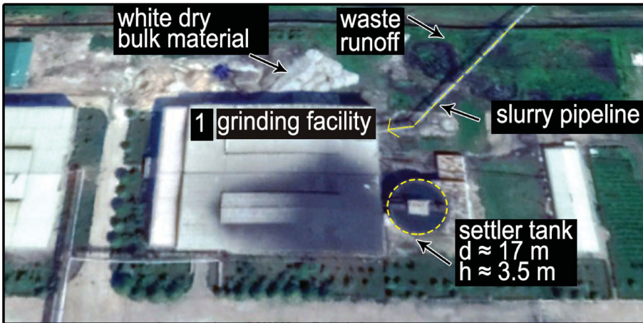
Figure 6. A probable grinding facility. This is the first building to which slurry is transported to. Source: Google Earth.
