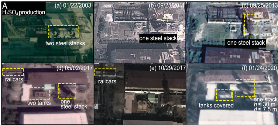
Figure 15. (a–f) A facility that is presumably used for production of sulfuric acid ( \text{H}_2\text{SO}_4 ) over time. Satellite images show construction of two tanks in 2017, in addition to disassembling of one steel stack. Source for a–d, f: Google Earth. Source for e: Copyright MAXAR 2021; Image credit: Apollo Mapping.
