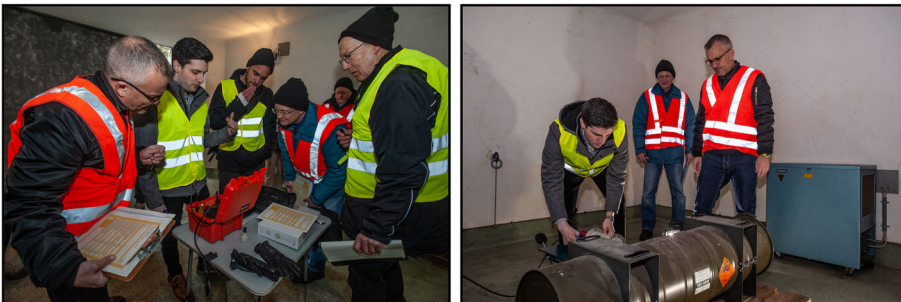
Figure 3. Participants of the Menzingen Verification Experiment. Left: Host (yellow vests) and inspector (orange vests) teams discussing the operation of the Absence Confirmation Experimental (ACX2) device. Right: Participants set up the sodium iodide detector for passive gamma ray and transmission measurements of the inspected container. Source: Pavel Podvig.
